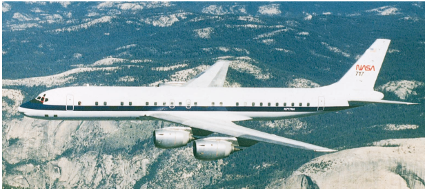
FIGURE 14. The NASA/Jet Propulsion Laboratory AIRSAR aircraft containing the UHF, L-band, and C-band SAR radars. This aircraft was used to measure and characterize radar attenuation and backscatter caused by foliage in heavily forested areas.
