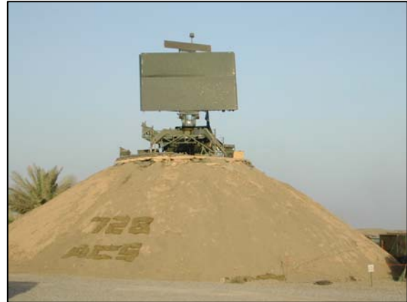
Radar "A" set up on abandoned Iraqi SA-9 mound.
