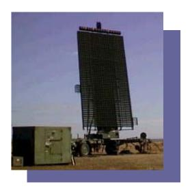
erected. The antenna operates in the 1215–1400 MHz frequency range, mechanically rotating at either a 5-second or 10-second rate to provide a 360° azimuth scan. The elevation scan is accomplished by electronic beam steering from 0° to 19° for ABT surveillance and up to 60° for TBM tracking.
