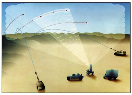
Firefinder is an integrated radar system that detects and tracks hostile mortar rounds, artillery shells and rockets, instantaneously locating their source.
