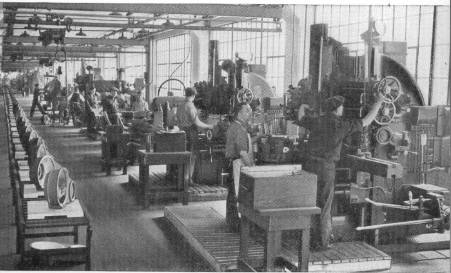
The elevation housing machine line. Machine tools in the foreground are boring mills.
