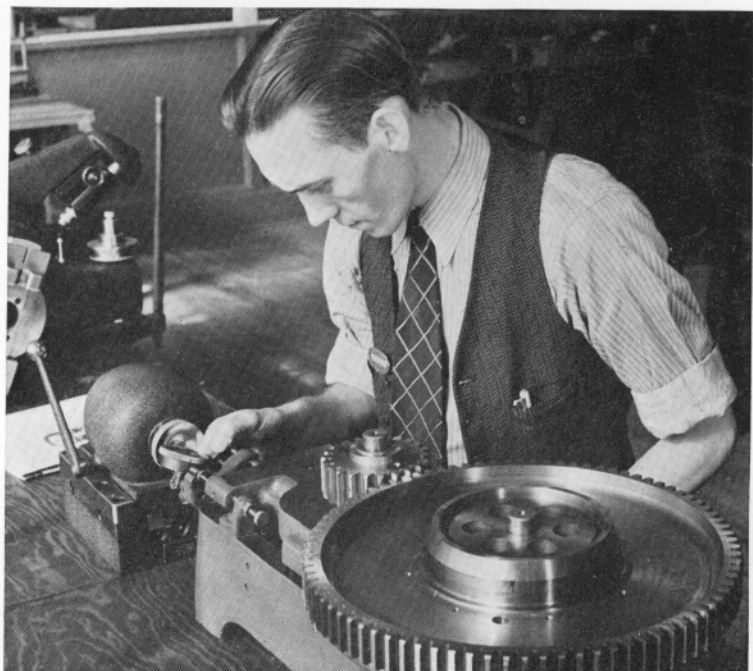
Inspector gauging the large 14½-inch gears which move the radar "dish" as it scans the heavens.
