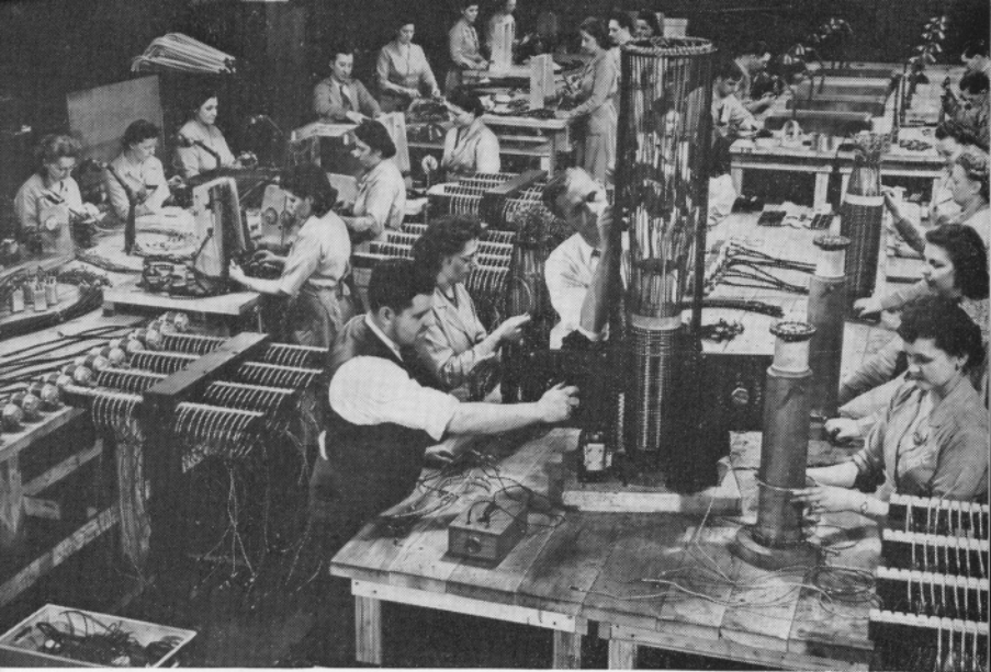
Women did most of the assembly of the slip rings and wiring of the main drive shaft.
