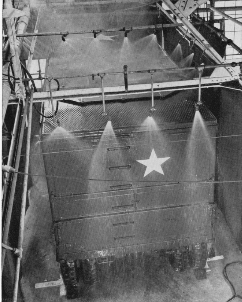
Each semi-trailer was put through a high pressure shower bath to test the tightness of its joints against rain.
