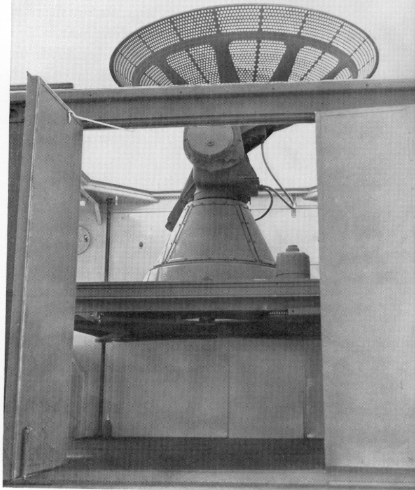
When put into use, the SCR-584 radar is raised through a trap door. Side panels are opened to show the process.
